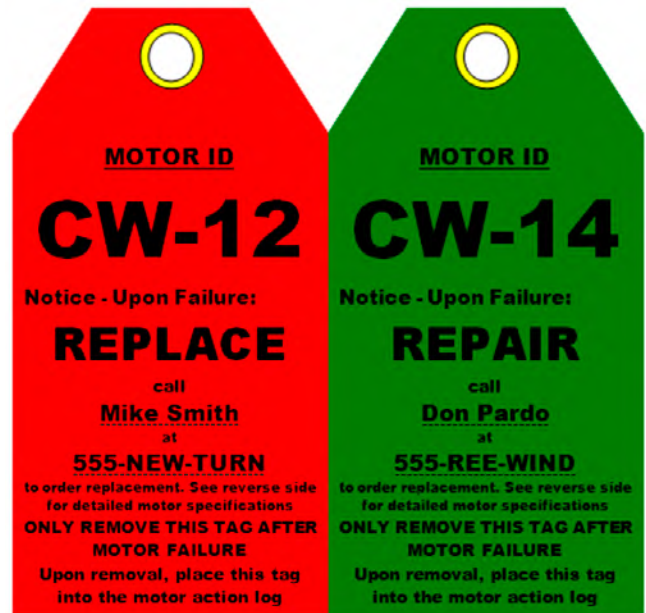
Figure 7-6. Sample In-Service Motor Repair/Replace Tags. Tags from Advanced Energy
